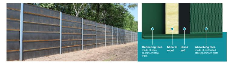
Gramm Barriers METASoundBlok® Corten are made from CORTEN steel to help it blend in with more rural sites with natural green, brown or orange colours. The panels also look stunning with urban environments creating a striking feature wall. The inside of the Metal panel is made up of sound absorbing mineral wool to achieve an A5 noise reduction rating.
