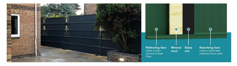
Gramm Barriers METASoundBlok are made from DX51D+Z200/275-NA grade galvanised steel plating which can be powder coated to any shad of RAL colour. The panels can also be finished in a galvanised finish or CORTEN to help it blend in with more rural sites. The inside of the Metal panel is made up of sound absorbing mineral wool to achieve an A5 noise reduction rating.
