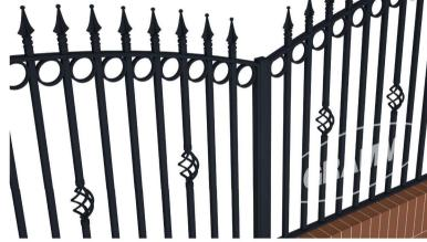
Featuring steel 12, 16, 20 & 22 Diameter of round or side of square vertical railings set at 112mm & 120mm centres. Security fixings are used fastening each panel to the galvanised 50 x 50mm, 70 x 70 or 80 x 80mm RHS steel posts, this railing system is built to last. (100 x 55mm RSJ post also available) ArmaBarDESIGNER® provides a bespoke service to satisfy individual needs in terms of product type, size, finish and features. The ArmaBarDESIGNER® complements all our railing systems.
