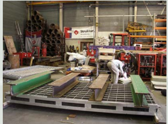
Windload test for NS-Railway
